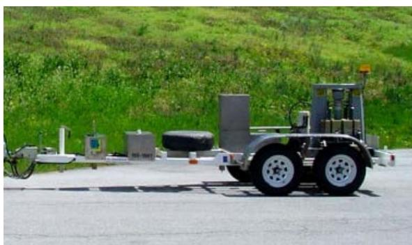
3-rasm. FWD (Falling Weight Deflectometer)ning umumiyo ko’rinishi.
